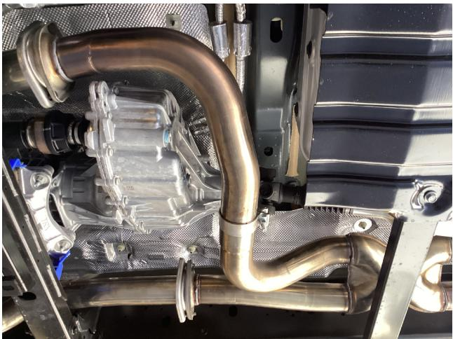
**Step 3:** Begin installing your new system by first loosely attaching the Inlet Pipe Assembly to the catalytic converter outlet flange using the supplied hardware. Next, attach the X-Pipe Assembly by slipping the Inlet Pipe Assembly outlet to the X-Pipe Assembly inlet. Loosely secure using the supplied clamp. loosely attach the X-Pipe Assembly inlet flange to the catalytic converter outlet using the supplied hardware.
