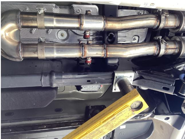
**Step 4:** Loosely install the Mid Pipe Assemblies by attaching the inlet ends to the outlets of the X-Pipe Assembly. The Pipe assembly with the welded hanger goes on the passengers side. Locate the welded hanger to the rubber insulator.
