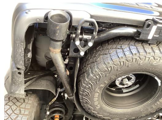
**Step 7:** Loosely install the two Tailpipe Extension Pipes using the supplied clamps, Then Loosely attach each Tail Pipe Assembly to the Tailpipe Extension Pipes using the supplied clamps. Locate the welded hangers to the rubber isolators.
