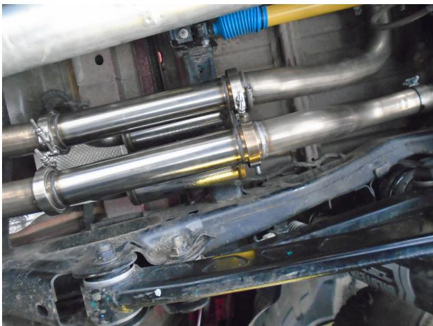
**Step 5:** Attach the Speq Resonator Assemblies to the Mid Pipe Assemblies using the supplied clamps
