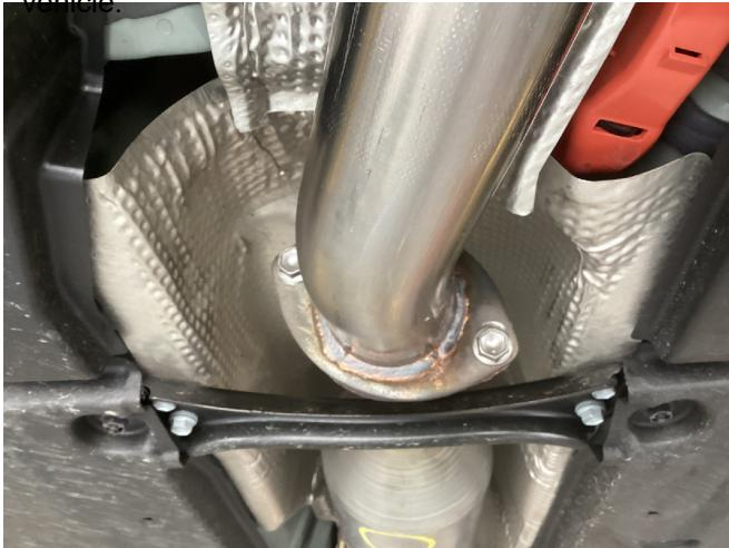
**Step 2.** Install Inlet Pipe Assembly. Loosely fasten it to the OE flange using the supplied fasteners and fit the hanger into the rubber insulator.
