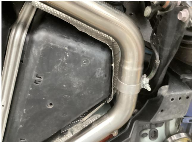
**Step 3.** Slide the Midpipe onto the inlet pipe and loosely secure using the supplied clamp.
