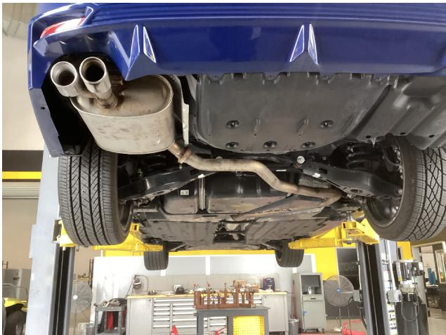
**Step 1.** Working front to rear loosen or remove all fasteners and clamps and disengage all welded hangers from the rubber insulators. Do not damage or discard the rubber insulators as they will be needed to install your new MAGNAFLOW system. Slide the OEM system off towards the front of the vehicle.
