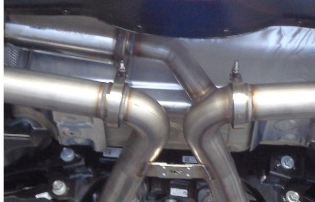
**Step 3.** Begin installation of the MagnaFlow system by attaching the Inlet Pipe Assembly to the downpipe using the supplied 3.20" clamp and re-using the OE fastener to attach the bracket. Next, attach the Y-Pipe Assembly using one of the supplied V clamps and engaging the hanger into the rubber insulator. (Leave all clamp and fasteners loose for final adjustment of the complete system.)
