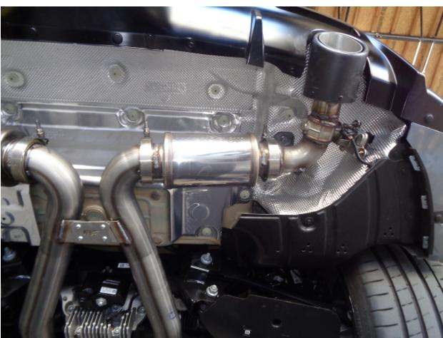
**Step 5.** The Tip Assemblies are attached to the Muffler Assemblies. Loosely attach the Drivers Side Tip Assembly to the Drivers Side Extension Assembly using the supplied V-Clamp. Loosely attach the Passengers Side Tip Assembly to the Passengers Side Extension Assembly using the supplied V-Clamp. Finish the installation by loosely attaching the MagnaFlow bracket between the Extension Pipes. Re-attach the valve wiring and OE cross brace.
