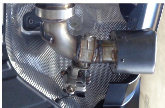
**Step 1.** To remove the OEM system first unplug the electrical connector at the exhaust valve located on the passenger side Tail Pipe. Begin by removing the cross brace then unbolt the mounting bracket and loosen the clamp at the exhaust inlet. Remove all welded hangers from the rubber insulators and remove the exhaust. Do not damage the fasteners or rubber insulators as they will be used to install the new MagnaFlow system.
