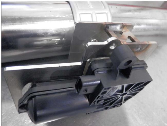
**Step 3:** Once the OEM exhaust system has been removed undo the three nuts attaching the exhaust valve motor to the valve and remove it. Before installing your new exhaust system attach the OEM valve motor to the MagnaFlow valve using the supplied hardware. The alignment spring on the motor will need to be engaged into the keyway slot of the new valve.
