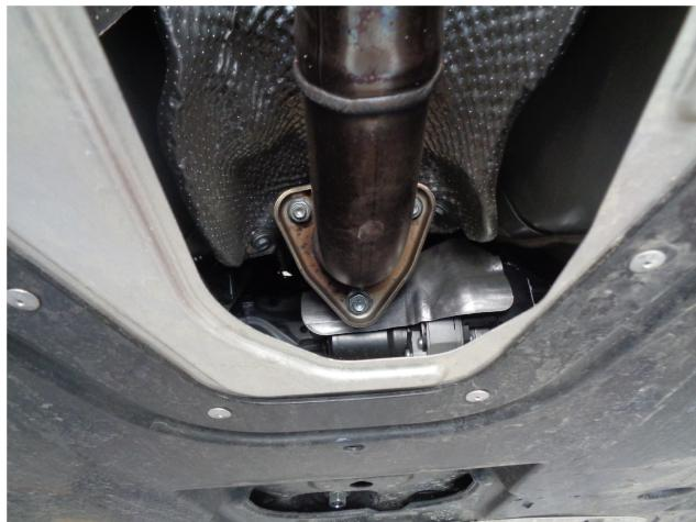
**Step 2:** To remove the OEM system first unbolt and remove the cross member at the inlet. Next, unbolt the inlet pipe at the catalytic converter flange junctions. Working front to rear disengage all welded hangers from the rubber insulators. The OE exhaust system can now be removed in one piece. Be sure to retain all mounting hardware as it will be needed to install your new MagnaFlow system
