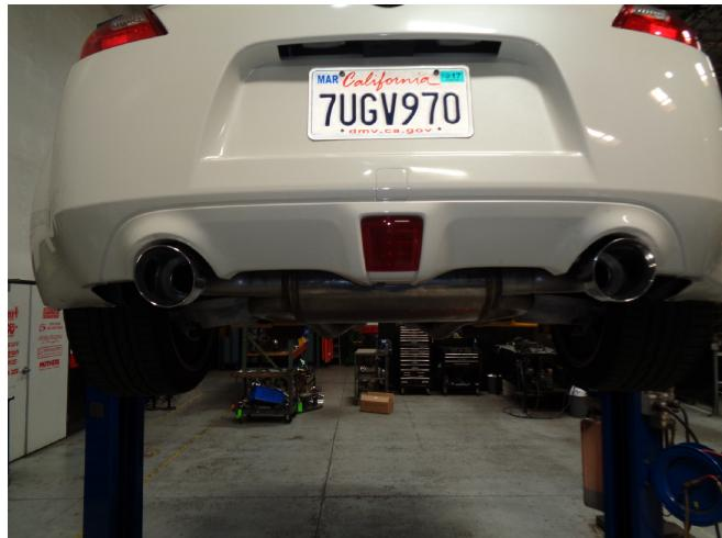
**Step 7.** Once a final position has been chosen for the new exhaust system, evenly tighten all clamps and fasteners from front to rear using the torque specifications on page one of these instructions. Inspect all fasteners after 25-50 miles of operation and re-tighten as necessary.
