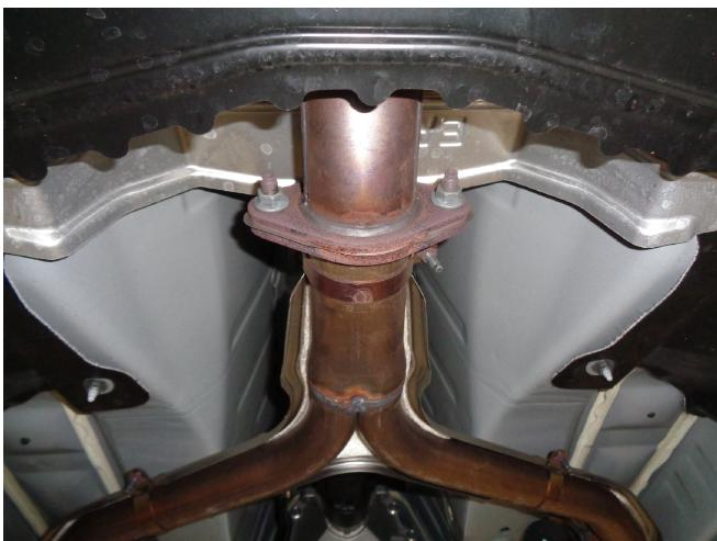
**Step 2.** Unbolt the flange coupling the inlet pipe assembly to the resonator assembly to ease the system removal process. Working front to rear disengage all welded hangers from the rubber insulators. Retain all mounting hardware as it will be needed to install your new MAGNAFLOW system.
