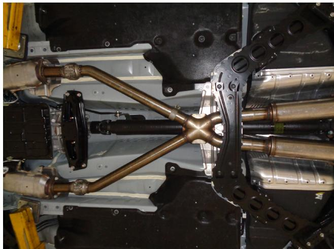
**Step 3.** Loosely install the new Inlet Pipe Assembly to the X-Pipe Assembly with the supplied clamp. Next, loosely bolt both inlet flanges to the catalytic converter outlets using the OEM gaskets and
