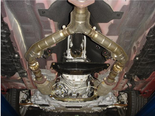
**Step 1.** Begin removal of the OEM exhaust by unbolting the inlet pipes from the catalytic converters at the flange junctions.
