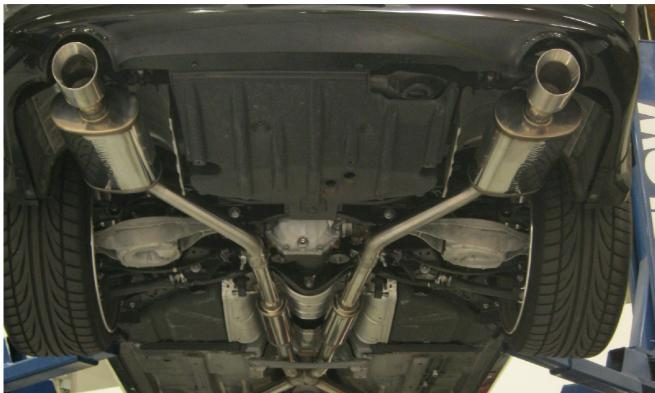
**Step 5.** Install both Muffler Assemblies by loosely attaching the inlets to the Resonator Assemblies outlets using the supplied clamps. Locate the welded hangers to the rubber insulators. Loosely secures using the supplied clamps.
