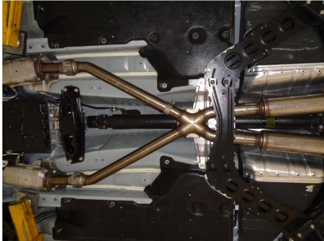
**Step 3.** Loosely install the new Inlet Pipe Assembly to the X-Pipe Assembly with the supplied clamp. Next, loosely bolt both inlet flanges to the catalytic converter outlets using the OEM gaskets and fasteners.
