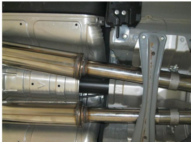
**Step 4.** Next, loosely attach both Resonator Assemblies to the X-Pipe Assembly outlets using the supplied clamps. Locate both welded hangers to the rubber insulators.
