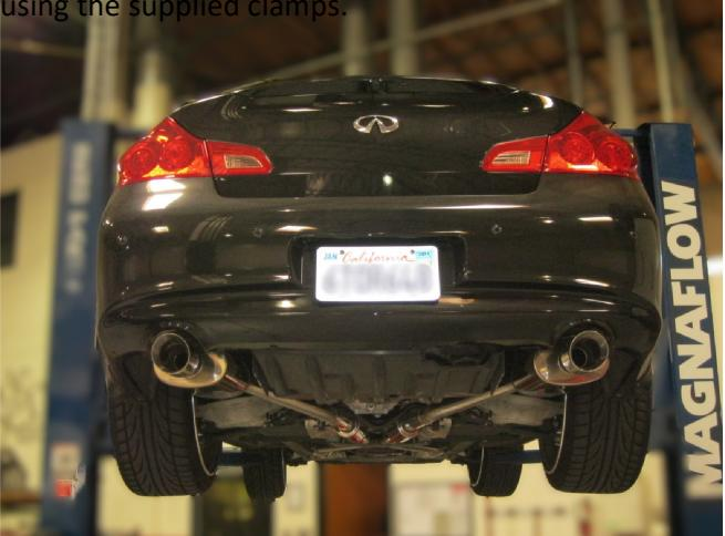
**Step 6.** Once a final position has been chosen for the new exhaust system, evenly tighten all clamps and fasteners from front to rear using the torque specifications on page one of these instructions. Inspect all fasteners after 25-50 miles of operation and re-tighten as necessary.
