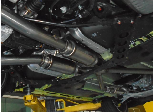
**Step 5.** Loosely fit the supplied 5x11 Resonators to the flange ring outlet of the X-Pipe Assembly
