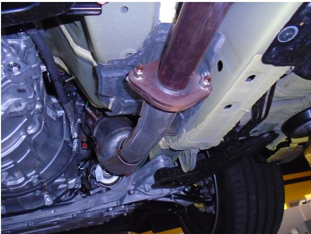
**Step 1.** Begin removal of the OEM exhaust by un-fastening the inlet pipes from the catalytic converters at the flange junctions.
