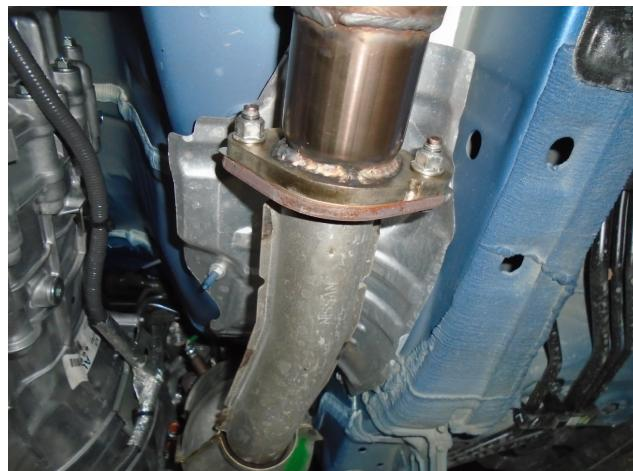
**Step 3.** Begin installing the new exhaust by loosely attaching the Inlet Flex Assemblies to the catalytic converter outlets using the OEM gaskets and fasteners
