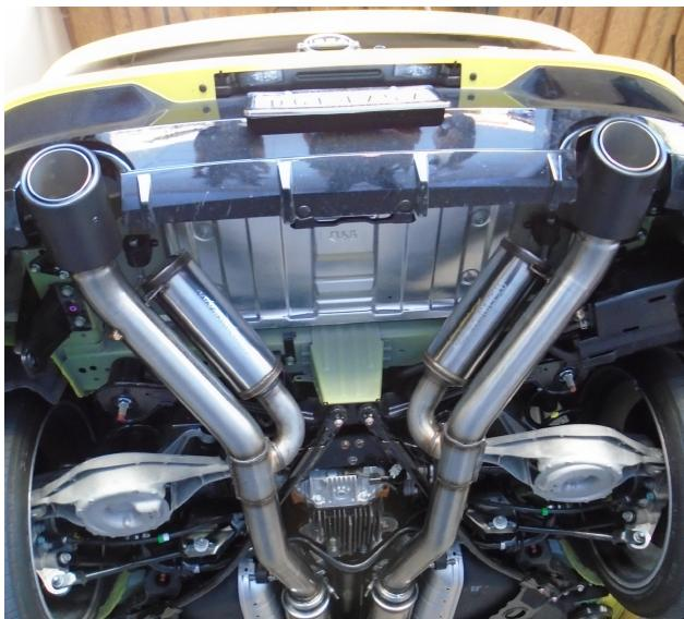
**Step 6.** Install the Resonator Assemblies using the supplied V-Band clamp. Attach the welded hangers to the rubber insulators and position the tips into the rear valance.
